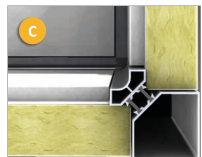
60 mm thermal break profile 63 mm thickness profile
